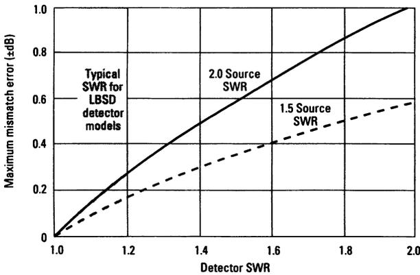
Figure 4. Measurement uncertainty due to detector source mismatch.
