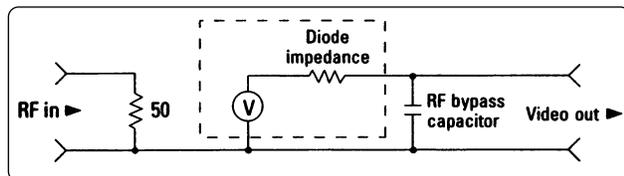
Figure 7. Detector equivalent circuit.
